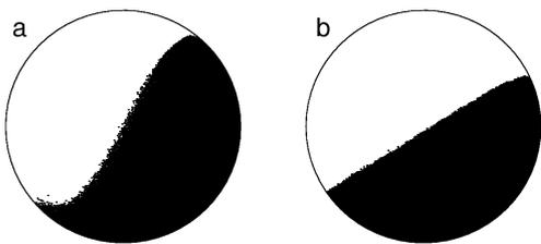
FIG. 2: Side views of the 3D drum. In both cases,  $R = 80d$ ,  $L = 10d$ ,  $\mu = 0.3$ ,  $\Omega=0.1$  rad/s and  $N=36\,000$  grains. a) frictional and b) frictionless end plates. The difference in shape is very clear and originates from a change in the frictional properties of the end plates. This provides evidence of the crucial role of the end plates on the shape of the free surface.
