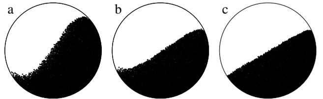
FIG. 4: Side-views of the 3D-drum. In all cases,  $R = 40 d$ ,  $\mu = 0.3$ , and  $\Omega=0.2$  rad/s. a)  $L = 10 d$ , b)  $L = 50 d$ , c)  $L = 300 d$ . The longer the channel, the flatter the surface. This result gives further support to the idea that the end plates are responsible for the S shape of the free surface.
