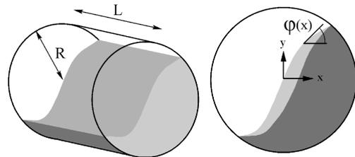
FIG. 1: We consider a half-filled three dimensional drum of radius  $R$  and length  $L$ . The local slope of the free surface is denoted  $\varphi(x)$ . Right: light grey corresponds to flowing material and dark grey to solid rotation.
