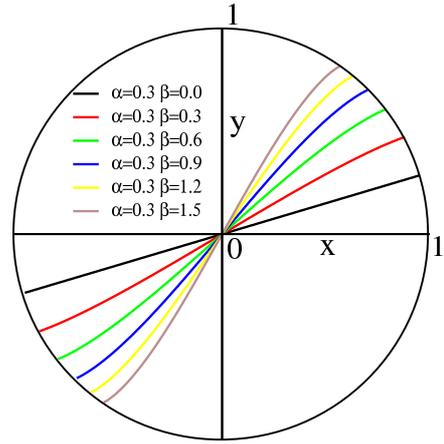
FIG. 3: (Color online) Numerical solutions for  $y_{surf}$  for  $R = 1$ ,  $\mu_i = \alpha = 0.3$  and various values of  $\beta = \mu_w/L (d\Omega^2/g)^{1/4}$ . For  $\beta = 0$ , the influence of the end plates is null and the free surface is flat. When  $\beta$  is increased, i.e. increasing influence of the end plates, a curvature appears and the free surface displays an S shape.
