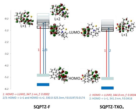
Figure 4. The first calculated electronic transitions of **SPQZT-F** (Left) and **SPQZT-TXO<sub>2</sub>** (Right) by TD-DFT B3LYP/6-31G(d), shown with an isovalue of 0.04 [ $e \text{ bohr}^{-3}$ ]<sup>1/2</sup>.
