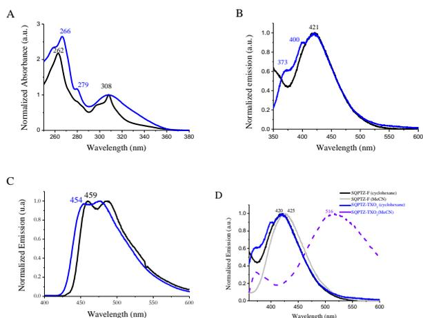
Figure 3. Optical properties of **SPQZT-F** (black line) and **SPQZT-TXO<sub>2</sub>** (blue line); **A**: UV-vis absorption spectra (cyclohexane), **B**: Emission spectra (cyclohexane) at rt under argon ( $\lambda_{\text{exc}}=330$  nm), **C**: Emission spectra at 77K (2-MeTHF,  $\lambda_{\text{exc}}=315$  nm). **D**: Emission spectra in cyclohexane and acetonitrile.
