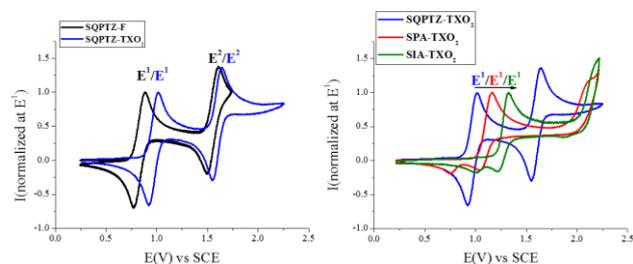
Figure 2. Cyclic voltammetry ( $\text{CH}_2\text{Cl}_2 + \text{Bu}_4\text{NPF}_6$  0.2 M, sweep-rate 100  $\text{mV}\cdot\text{s}^{-1}$ ) of **SQPTZ-F** and **SQPTZ-TXO<sub>2</sub>** (left) and **SIA-TXO<sub>2</sub>**, **SPA-TXO<sub>2</sub>** and **SQPTZ-TXO<sub>2</sub>** (right).
